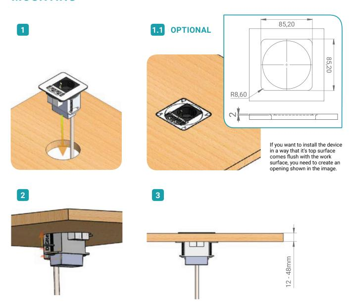
It is easily mounted in a Ø80 + 0,5mm opening with an integrated tightening mechanism and using only a PH screw driver. For desk thicknesses from 12 to 48mm.
